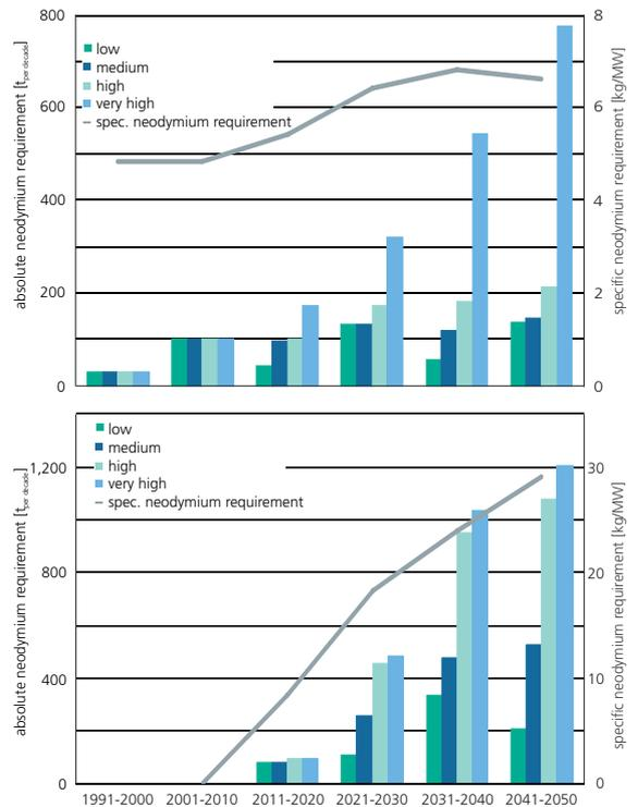
Figure 6: Neodymium requirement for new onshore (top) and offshore (bottom) wind turbines installed in Germany in the "Continuity" roadmap (specific and absolute, for each decade in each case)
