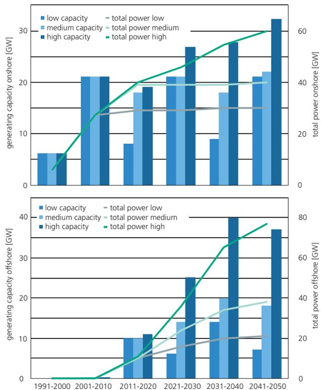
Figure 2: Overall capacity at the end of a decade and capacity expansion per decade for the different expansion paths
