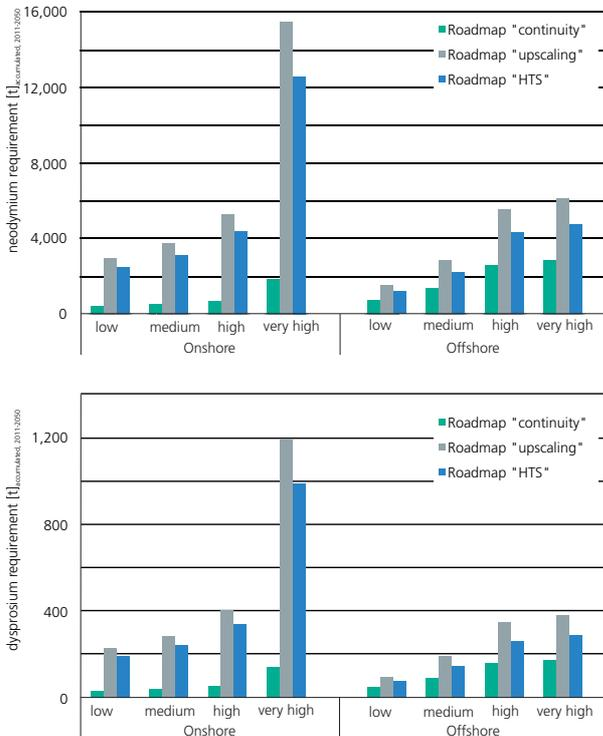
Figure 5: Cumulated neodymium (top) and dysprosium (bottom) requirement for new wind turbines installed in Germany between 2011 and 2050
