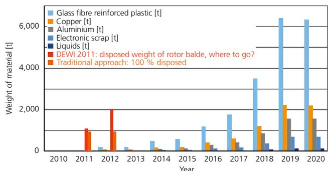
Figure 4: Estimated masses of materials from wind turbines [Albers et al. 2012]
