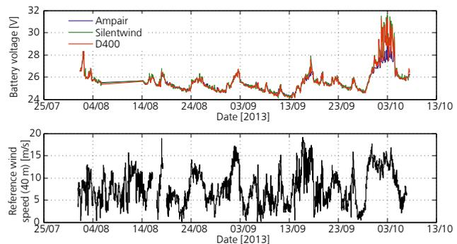
Figure 2: Transmitted status data (voltages of battery banks assigned to micro-WTs) during offshore test next to FINO1, in relation to reference wind conditions.
