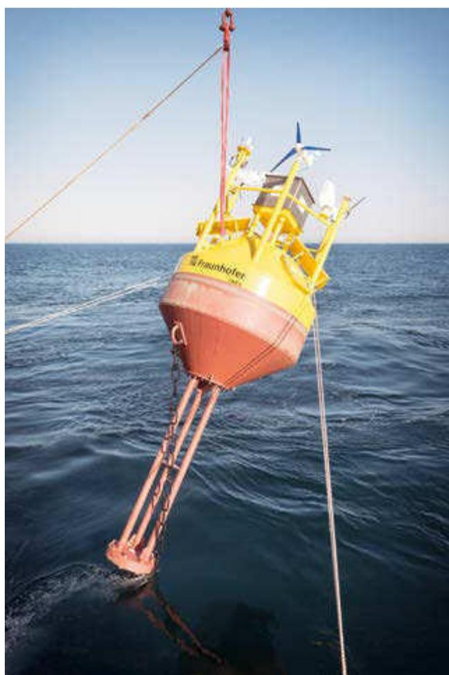
Figure 1: Fraunhofer IWES Wind Lidar Buoy before and during its first offshore trial. (Photographs: Caspar Sessler, Fraunhofer IWES)
