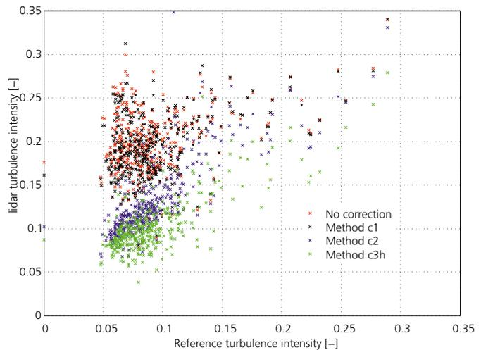
*Figure 5: Correlation between measured Turbulence Intensity (TI) from floating lidar and reference cup anemometers at 100 m measurement height for different correction approaches. Method c1 only considers the recorded yaw angles for the correction of the lidar data, c2 additionally the horizontal tilt angles, i.e. roll and pitch, and c3h in addition the heave of the buoy.*
